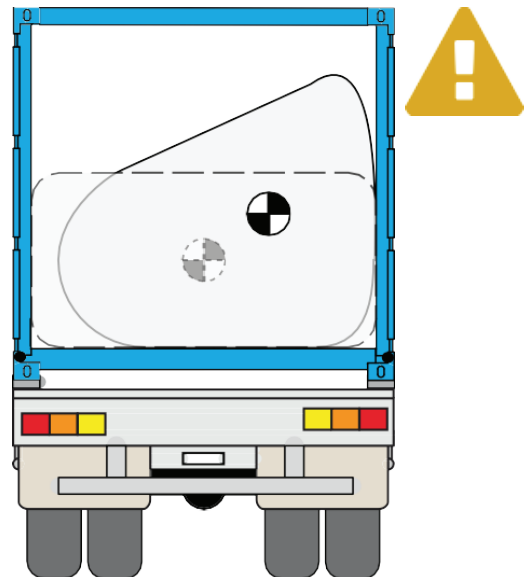
Flexible tank product surge
