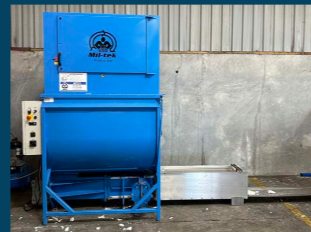
Polystyrene Compactor, Mainfreight 2Home Christchurch
