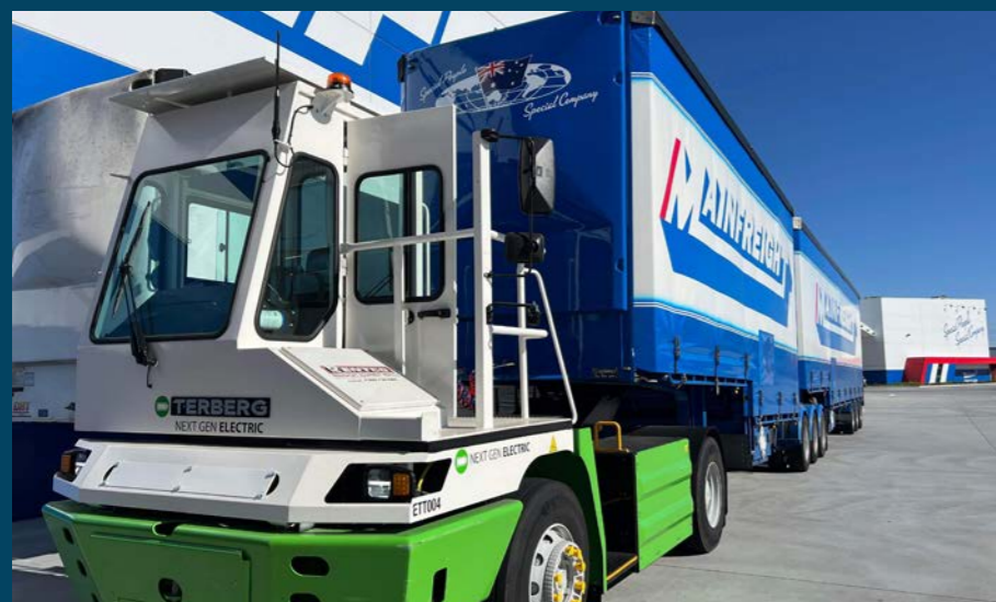
Electric yard truck, Dandenong South
